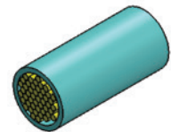
Duct containing 48 x Ø 1.2mm cable
