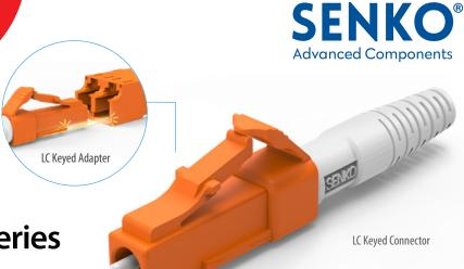
The SENKO LC Keyed Connector is a fiber optic connector that prevents improper connection of separate networks within common access points. It uses a patented keying system that allows only the same color connectors to mate with the same color adapters, ensuring that network segments are not accidentally mixed or crossed.
