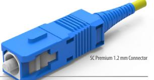
SENKO's SC Premium Connector 1.2 mm boot is based on the Senko Premium SC range and specifically designed to accept a reduced size, 1.2 mm cable that is commonly found in highly dense telecommunications cable racks and cabinets.
