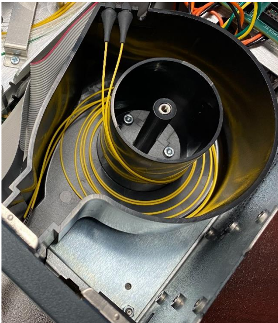
Figure 17: Exposed view of good output fiber management
