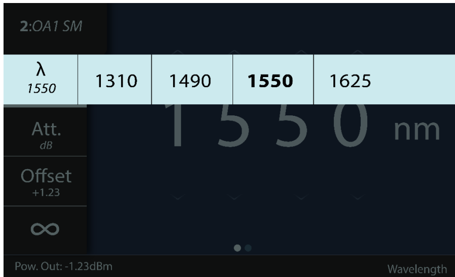
Figure 5: Front panel operation – wavelength flyout menu
