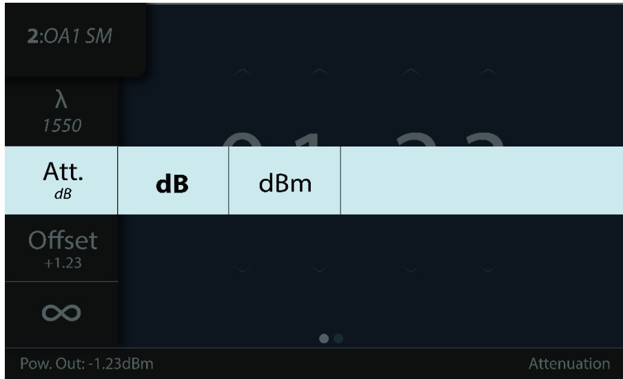
Figure 7: Front panel operation – attenuation flyout menu
