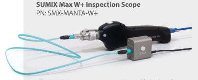
The MANTA W+ inspection scope is designed for high-performance inspection of all types of single fiber and multi-fiber optical connectors, patch cords and bulkheads. The MANTA HM inspection scope is used to detect scratches, contamination and other surface defects as small as 0.75  $\mu$ m on the end face of the connector.
