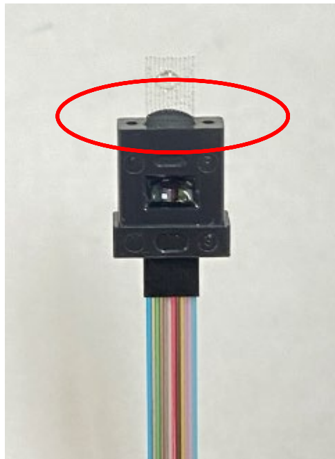
Figure 5 Proper epoxy amount
