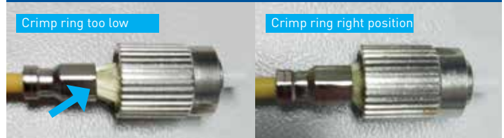
Figure 8: Improper crimp ring placement during crimping
