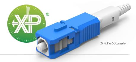
The XP Fit Plus° is a pre-polished, pre-assembled connector compatible with the standard SC connector. In place of epoxy, an internal mechanical grip gently but effectively holds the fiber in place and can be installed in under two minutes. Without polishing or adhesives, the XP Fit Plus° makes field installations quick and easy, eliminating the need for epoxy curing and hand polishing at the work site.
