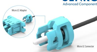
The SENKO Micro LC connector is designed to be compact, eliminating the need for finger access to the latch mechanism of traditional LC connectors. This allows LC adapters to be mounted much closer together than previously possible, maximizing space efficiency. Its small size combined with bayonet-style connectivity makes it particularly suitable for Behind-the-Wall (BTW) applications, where space constraints are critical.
