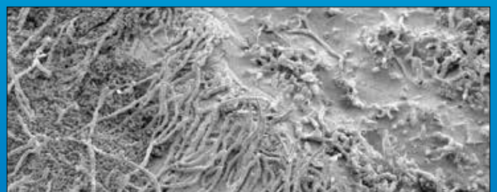
Flattening caused by degradation when using bad quality ferrules
