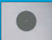
No ferrule roughening can be seen
