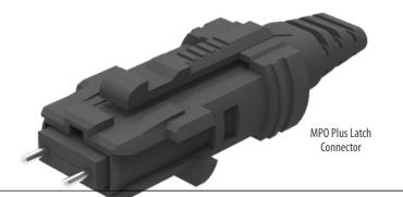
The MPO PLUS Latch connector features an innovative latch design for easier connection and disconnection than traditional push-pull MPO housings, while retaining the MPO Plus oval spring and free-floating high-quality ferrules. It is compact, with a 20N spring for 24F ferrules, and includes a high-quality, low-loss ferrule. Note that a latch-compatible adapter is required.
